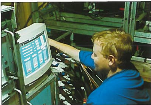
Above, screen tech Pete Egan at the OptiScreen's controls. Fibre-optic links are used between the control rack and LED panels; each panel has a separate fan power inlet to prevent condensation outdoors. Top right, the final result with the OptiScreen giving an added dimension to the ICC stage
